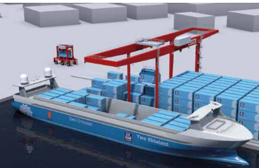
The Yara Birkeland , the world's first fully electric and autonomous container ship, is expected to start testing in 2020
